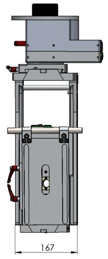
Weight 12.5 kg (27.5 lbs) 360 Deg in 2 Seconds (Pan & Tilt) Max. Load 35 kg
